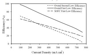
**Fig: 4(b).** Efficiency produced by SOFC/MGT at different current densities [14]
