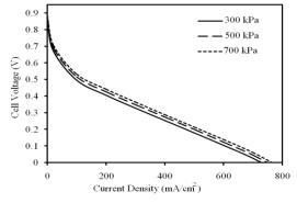
Fig: 3. Polarization Curve at Different Current Density [14]
