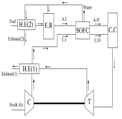
Fig: 1. Schematic Diagram of the Tubular SOFC/MGT Hybrid Power System [14] Table: 1. Specification of the hybrid SOFC/MGT system
